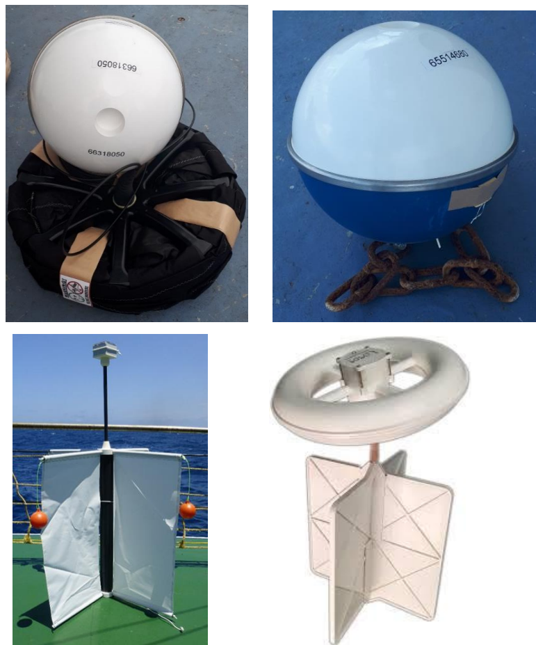
Fig. 1. Upper panels, from left to right: SVP (surface buoy with a holey-sock drogue) and DWS drifters (surface buoy with ballasting chain). Lower panels, from left to right: CODE and CARTHE drifters.
